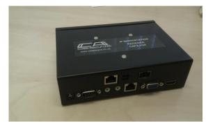
C.A. Designs Fibre **IP** extender systems enable IBM-compatible computers to be operated with the monitor remote from the system unit. Each **CX\*** or **VX\*** system comprises:
